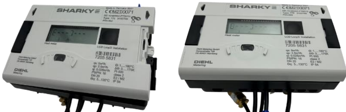
Figure 8 Closing the meter housing starting from left edge then closing the meter housing with the side latches
